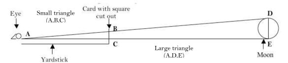
The distance between the card and the mark should be about  $55 \frac{1}{2}$  inches and the opening in the card is  $\frac{1}{2}$  inch. The distance to the Moon is about 240,000 miles.
